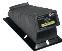
RCC-14 Remote Contactor and Current Control 151086 East/west rotary-motion fingertip control attaches to TIG torch using two hook-and-loop fasteners. Includes 26.5-foot (8 m) cord and 14-pin plug.
