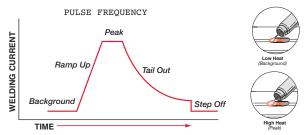
**Pulsed MIG Mode** varies weld current between peak (high heat) and background (low heat) current to provide better control of heat input, which minimizes warping and burnthrough on thin materials. Pulsed MIG also enables flat, horizontal, vertical up, or overhead welding without a slag system. Optimized GMAW-P waveforms are readily available to use on aluminum, carbon steel, high strength low alloy steel, stainless steel, and nickel alloys.
