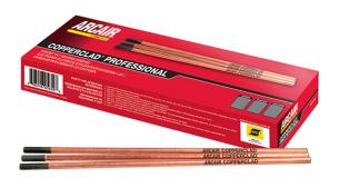
A high grade, all purpose copperclad pointed gouging electrode. It's controlled copper coating improves electrical conductivity (for more efficient, cooler operation) and helps maintain electrode diameter at the point of the arc.
