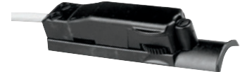
RCCS-14 Remote Contactor and Current Control 043688 North/south rotary-motion fingertip control attaches to TIG torch using two hook-and-loop fasteners. Great for applications that require a finer amperage control. Includes 26.5-foot (8 m) cord and 14-pin plug.
