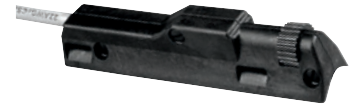
RCC-14 Remote Contactor and Current Control 151086 East/west rotary-motion fingertip control attaches to TIG torch using two hook-and-loop fasteners. Allows complete current and contactor control at operator's fingertips. Includes 26.5-foot (8 m) cord and 14-pin plug.
