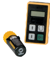
Wireless Remote Hand Control 300430 For remote current and contactor control. Receiver plugs directly into the 14-pin receptacle of Miller machine. 300-foot (91.4 m) operating range.
