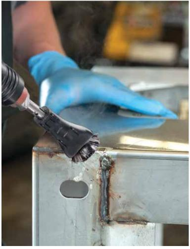
A highly effective method for removing heat tint from welded stainless steel without altering the surface of the parent material. SURFOX promotes the formation of a uniform and durable chromium oxide passive layer to protect stainless steel against corrosion.
