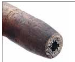
Nozzle fully clogged (not using E-Weld Nozzle)
