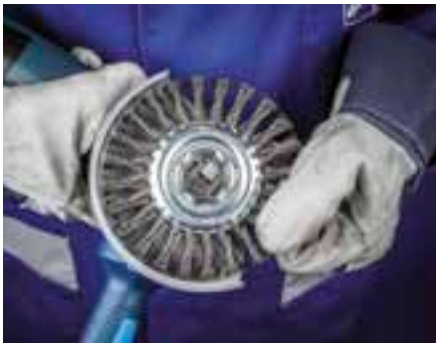
Place the brush on the X-LOCK holder in a form-fitting manner.
