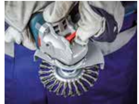
Release the brush by using the lever.
