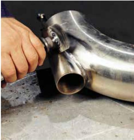
▷ Crimped wire for general surface cleaning, rust, scale and paint removal, etc.
