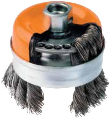
**Power brushes have long been used** for edge and surface conditioning on a wide variety of materials. Unlike grinding wheels and other abrasives that remove base material along with surface contaminants, power brushes work on the metal surface without removing the base material. The tips of the wire hammer the metal surface like thousands of tiny ball peens to finish and work the surface.
