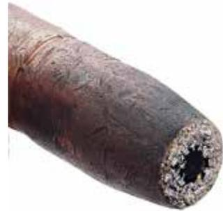
*Nozzle fully clogged (not using E-WELD Nozzle)*
