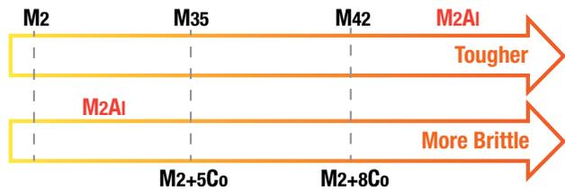
Adding Cobalt makes cutters more resistant to wear, but also more brittle which makes them more susceptible to breakage under pressure. M2Al provides an ideal blend of extreme toughness without a kind of “micro-flexibility” not found in standard cobalt blends.
