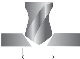
More metal to metal contact increases friction and heat, causing tooling to wear prematurely and resulting in longer cutting time
