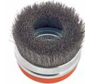
▷ *Safety supporting ring controls flaring to extend brush life. Once wires are worn down to the ring, the ring can be removed to expose more wire for extra brush life*
