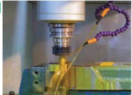
COOLCUT™ NEO 3724 N is a very high-performance cutting oil made from low emission base oils and effective EP-additives for severe cutting operations. Universally applicable for turning, milling, broaching, deep drilling, threading and more, this fluid is designed for use specifically on high tensile materials like high alloyed steels, Nickel- and Titanium-alloyed steels and stainless steels.
