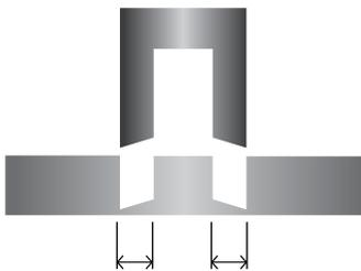
Less metal to metal contact reduces friction, reducing heat, increasing tool life and efficiency
