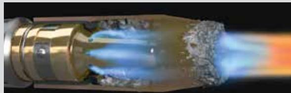
During the welding process, welding nozzles and tips get clogged with hot spatter which fuses to the nozzle, creating obstruction. This prevents the shielding gas to flow freely and heat the wire evenly.
